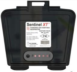
14 Rev. F gauge is on the back of the battery pack and has four LED lights and a push button to actuate the gauge. When the push button is actuated, LED lights are displayed which indicate the level of battery charge. If four (4) lights are illuminated, the battery is fully charged. If only one, two, or three lights are illuminated, more time is needed to charge the battery. Place the battery pack back in the cradle and wait until the charger LED turns green, fully charged, before using.
